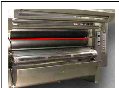
In-running nip: The red line shows a safety trip device to stop fingers being trapped
