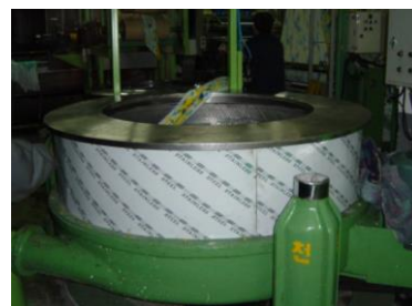
Hydro extractor with no lid: Poses an unacceptable risk to worker safety
